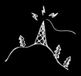
A signal from the base station meets the building envelope. The field strength outdoors is expressed in dBm, which indicates the decibel level relative to milliwatts (mW).
